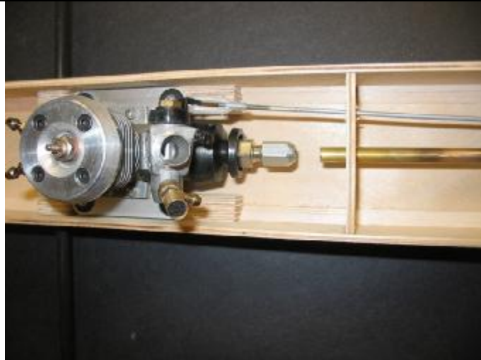
Nylon clevis used at metal throttle arm.
