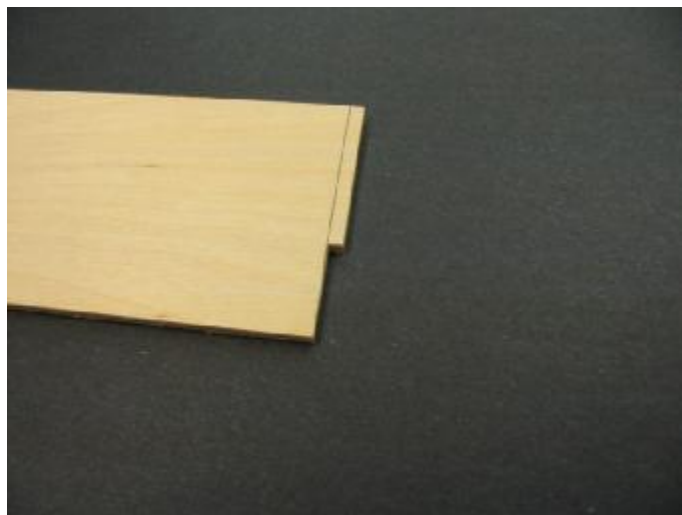
Tub side marked for transom alignment.
