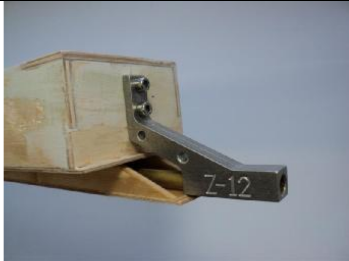
Strut sitting on ski with shaft tube cut flush.
