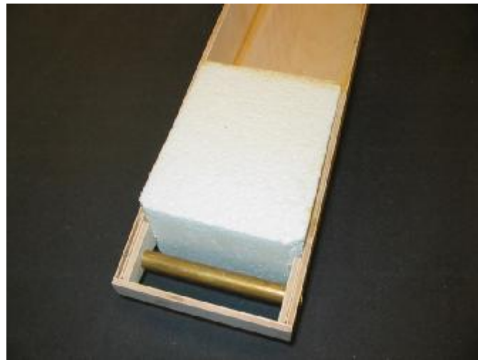
Foam nose block being test fit.
