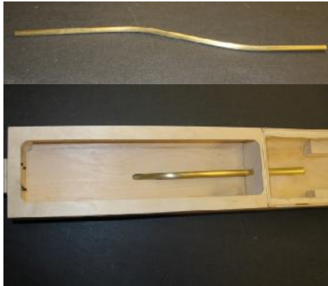
Shaft tube in place.
