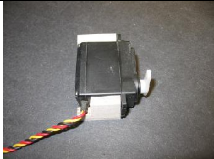
Side trimmed for servo wire clearance,
