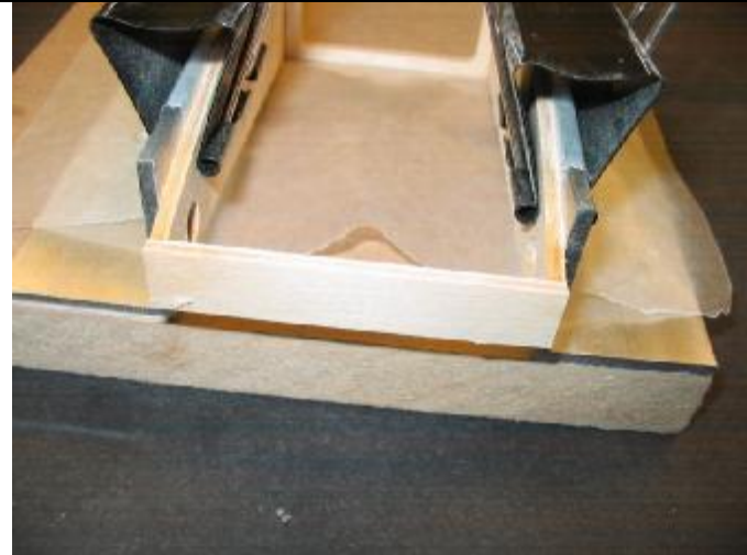
Tub sub nose being glued in place. Tub extends just past jig.
