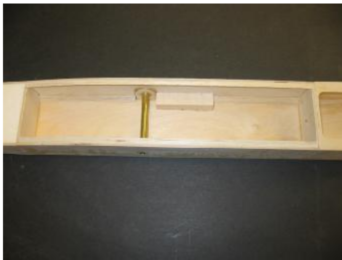
Engine rails glued in touching the aft doublers.
