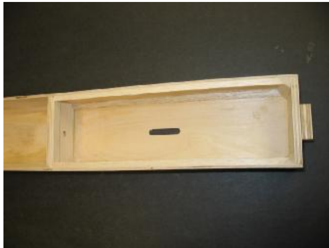
Upper tri stock in place. Note 5/16 tri on transom (servo mounts not shown). Block not used with Z strut.
