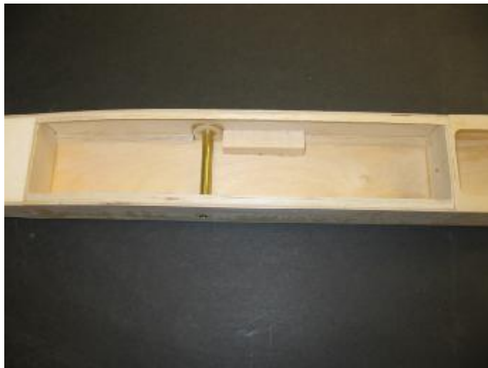
Engine bay with lower tri stock in place.
