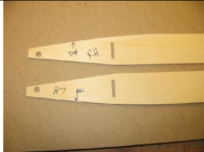
Tub sides marked before assembly.
