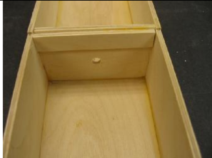
Radio box lid support glued in place behind bulkhead 2.
