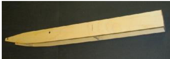
Tub sides glued to bulkheads.
