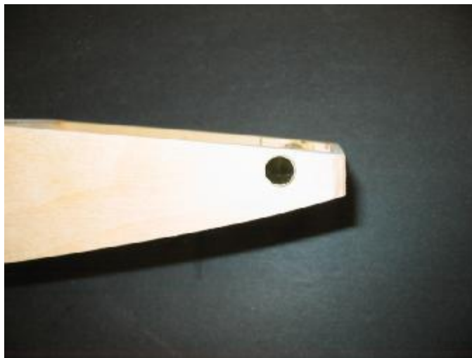
Tub sleeves sanded flush with tub side.
