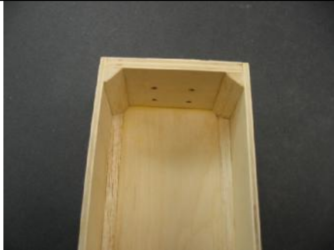
5/16 balsa tri stock transom reinforcement in place.
