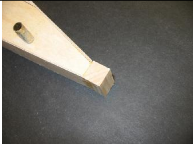
Pine sponson nose block in place.
