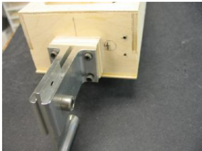
Rudder pushrod hole marked on transom.
