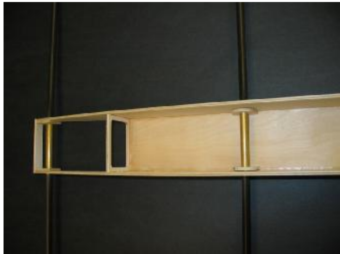
Tub sleeves, doublers and booms in place.
