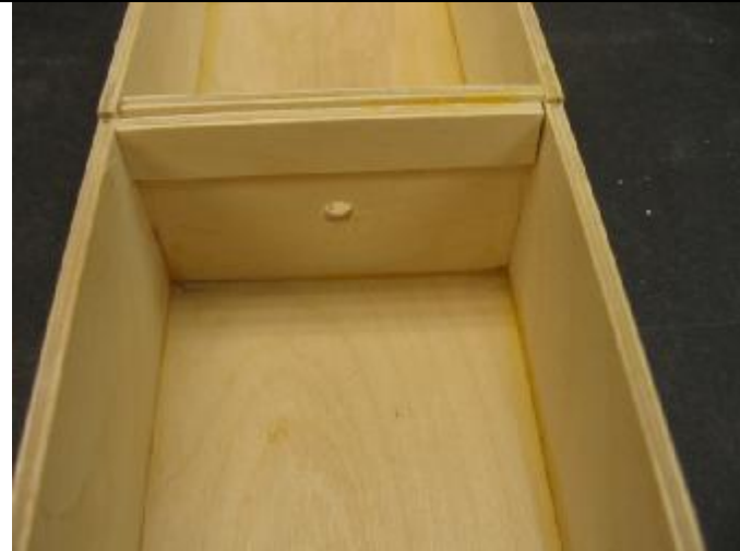
Radio box lid support glued in place behind bulkhead 2. 21 nitro shown. 21FE does not have step in sides.
