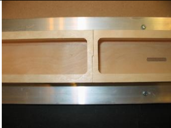
Forward and aft lid framed "keyed" to each other.
