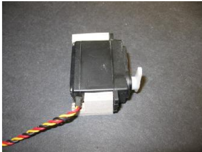
Side trimmed for servo wire clearance,
