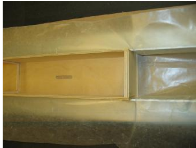
Waxed paper prevents one piece tub/jig assembly. 21FE shown.
