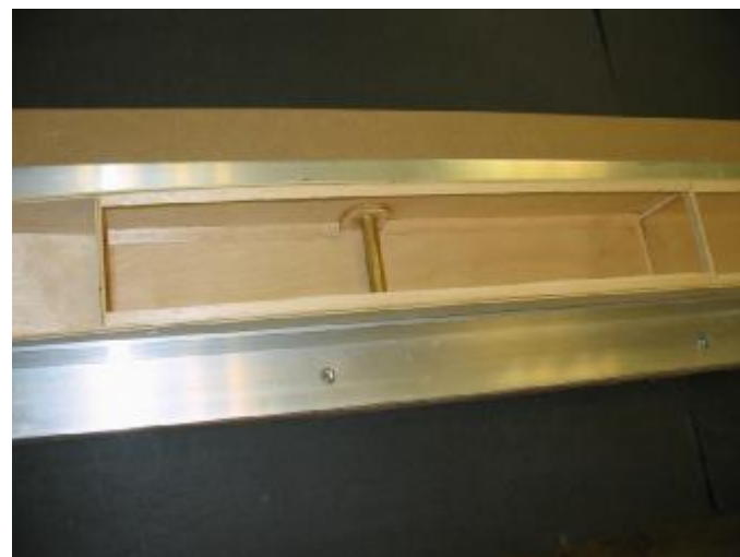
Balsa tri stock in place. See cutting guide in back of manual.
