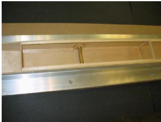
Upper balsa tri stock glued in place.
