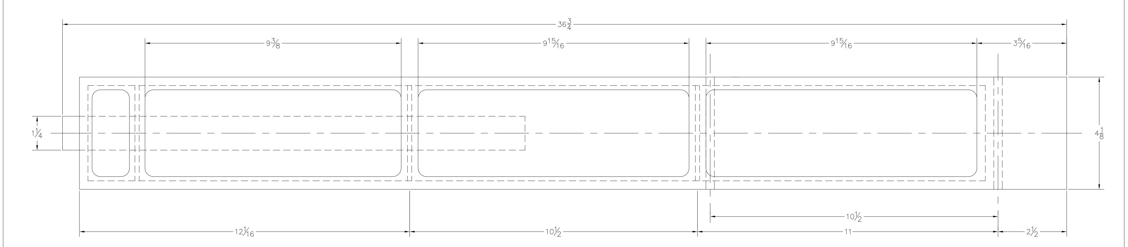
Add 1" of overall length to the back half of the tub for a 1.01 cid boat.
