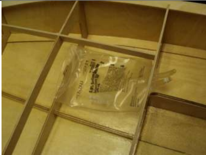
Mounting your fuel bag before the deck is on is easier.
