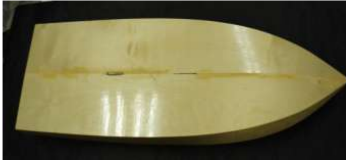
Hull with two coats of clear epoxy.
