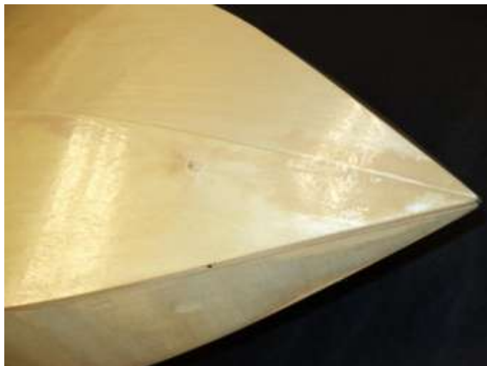
Hull sealed with epoxy.
