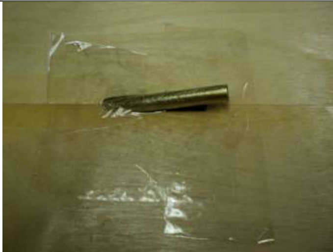
Tape applied to underside of stuffing tube,
