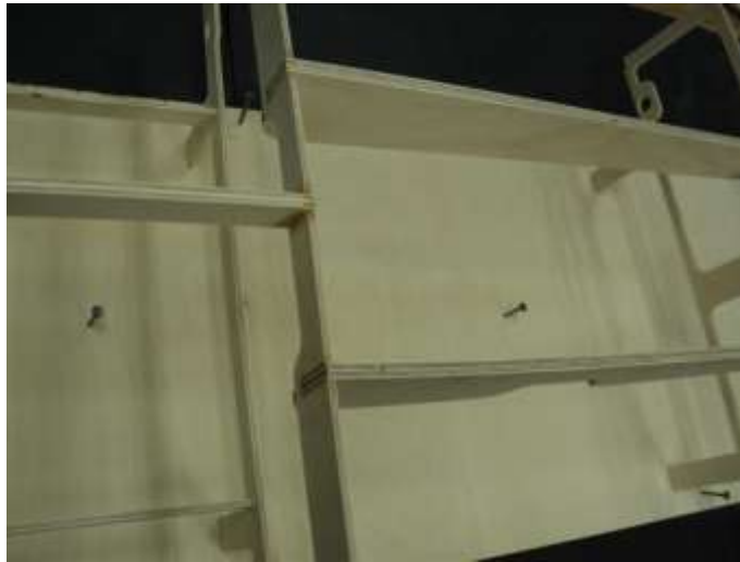
Keel and engine rails installed.
