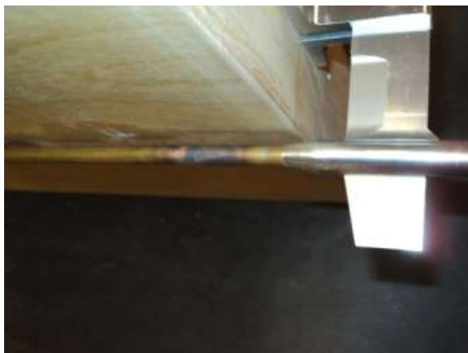
Rear portion of shaft tube annealed.
