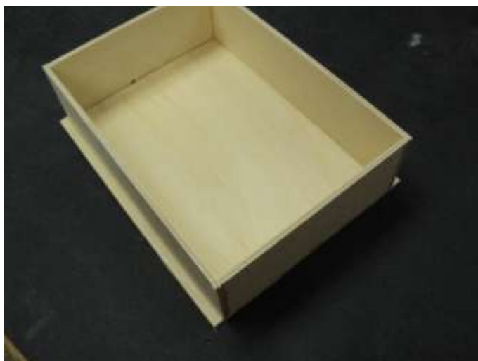
Bottom glued in place.
