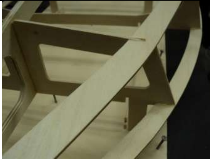
Install chines following angle of bulkhead.
