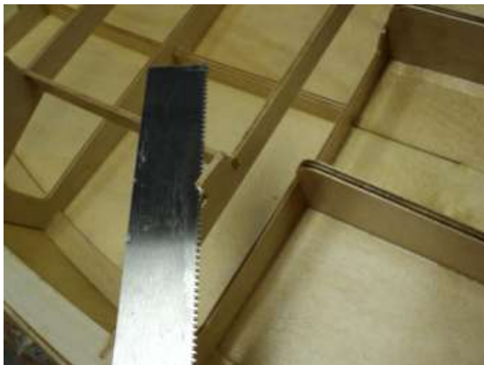
Trim building tabs. We love the flush cut saw for this.
