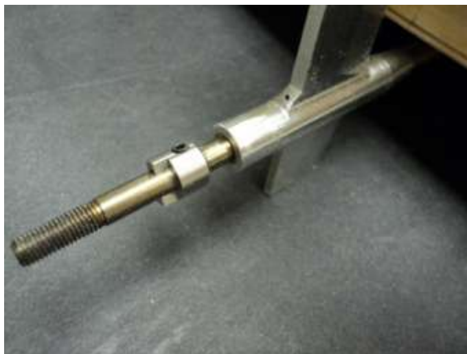
Leave a gap at the rear for flex shaft "wind up".
