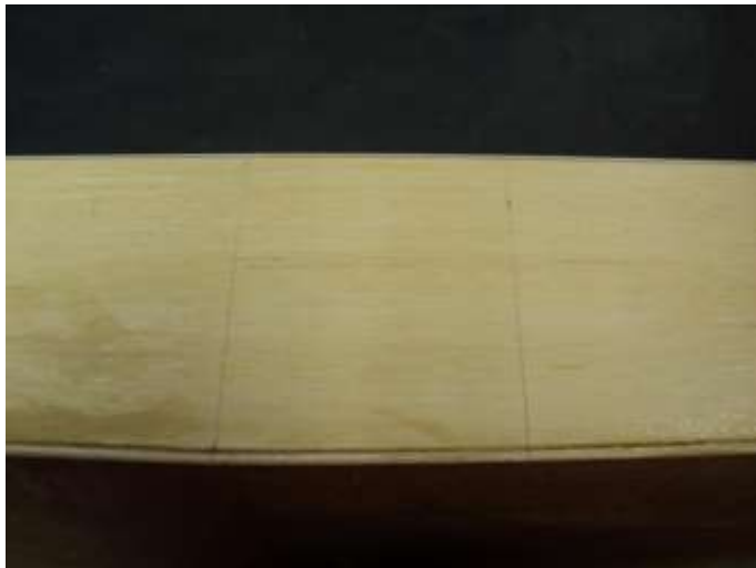
Center line and another mark 2-1/2 inches to the right.
