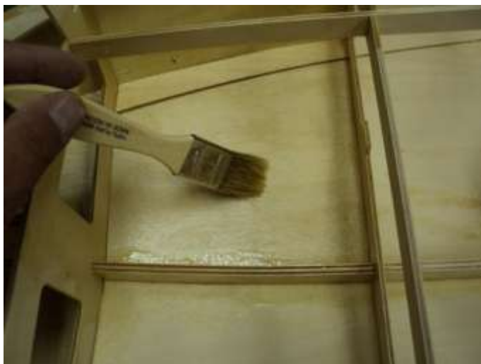
Sealing interior with epoxy.
