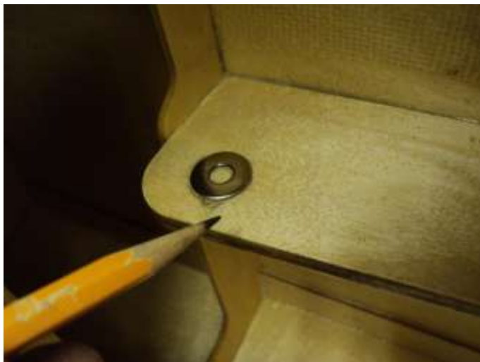
Tracing inside the washer for hole location.
