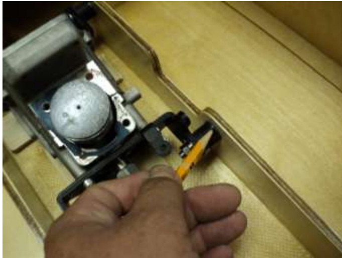
Marking the location of the rubber isolator.
