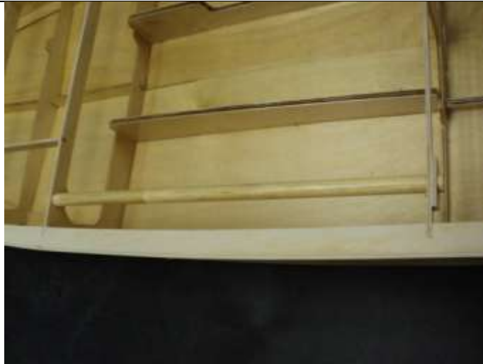
Deck support dowel glued in.
