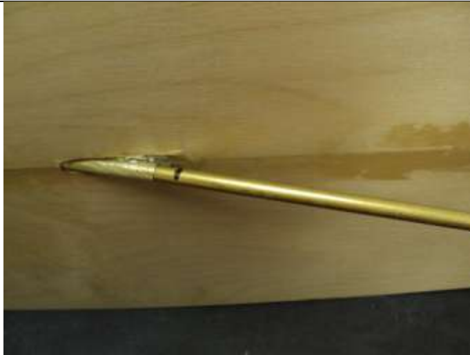
Marking exit of 5/16 shaft tube.
