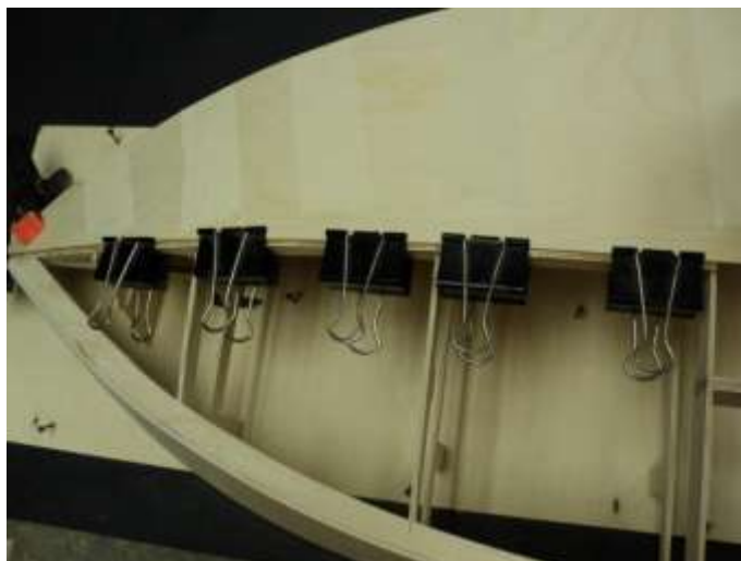
Bottom sheet taped and clamped in place.
