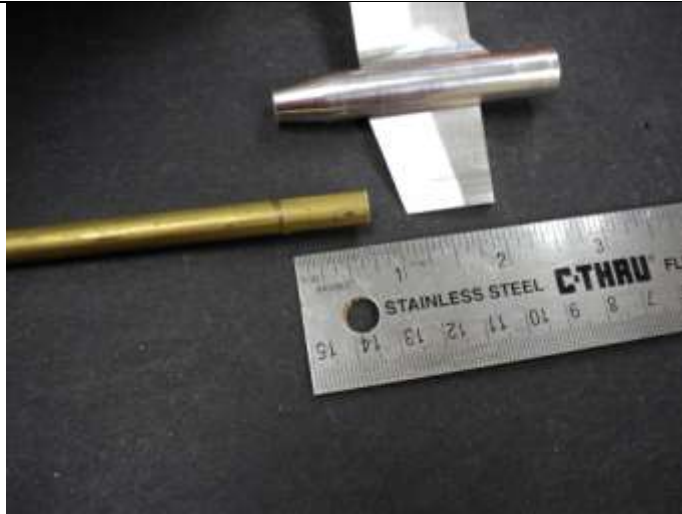
Marking depth of shaft tube inside strut.
