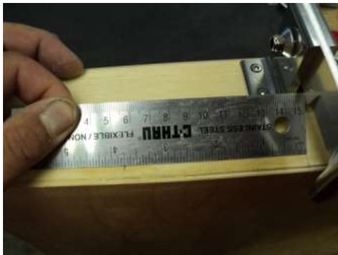
Measuring 3-3/4 from center for inside of trim tab.
