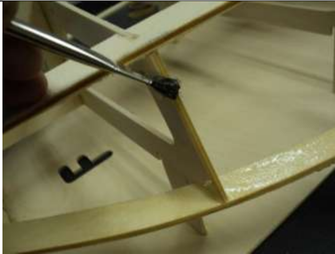
Brushing epoxy onto edges with cut down brush.
