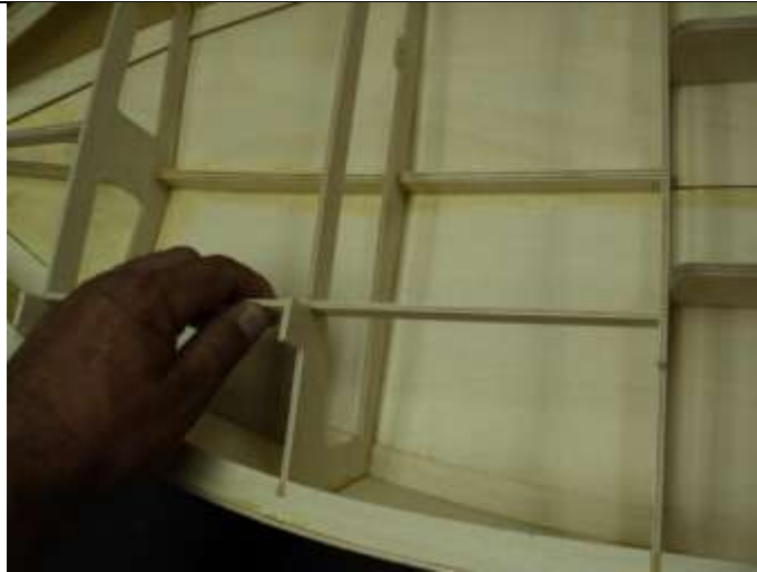
Installing spines. Hole goes forward.
