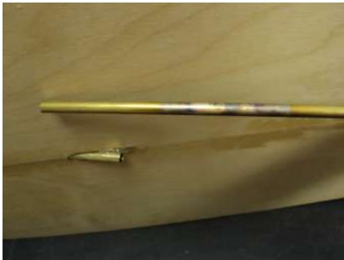
Shaft tube annealed.
