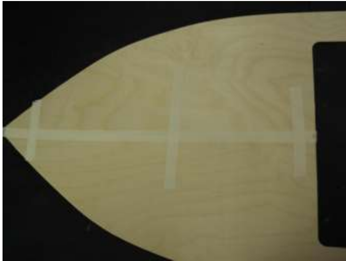
Top deck taped together until cured.
