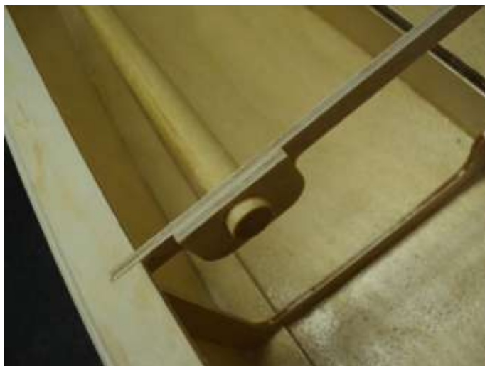
Aft dowel doubler detail.
