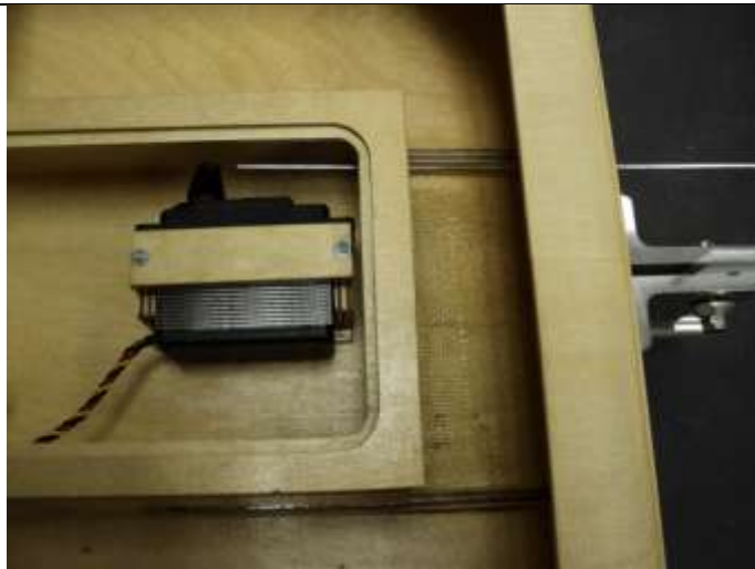
Rudder servo and pushrod in alignment.
