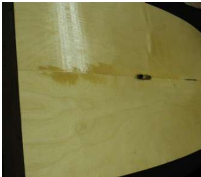
Hull sealed with epoxy.
