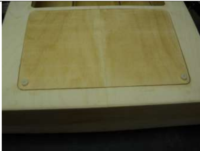
Hatch screwed in place.
