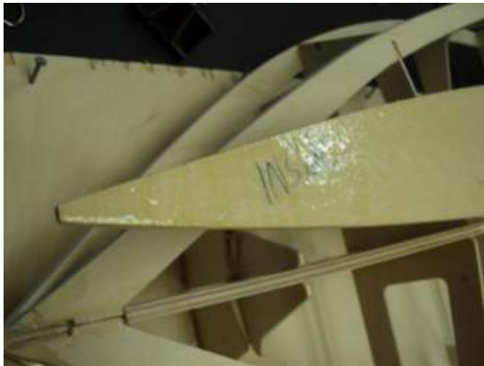
Front of side sheeting coated with epoxy.
