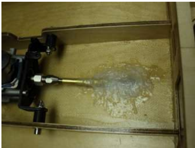
A strong shaft tube installation.
