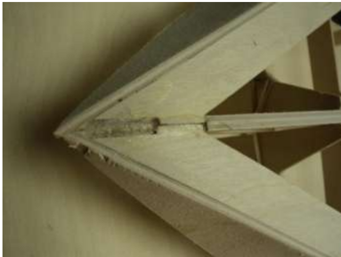
Side sheeting sanded flush at nose.
