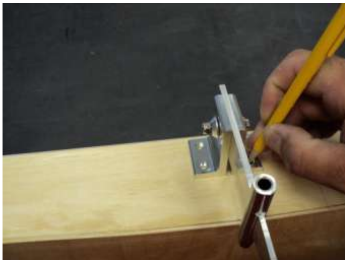
Marking strut holes in transom.
