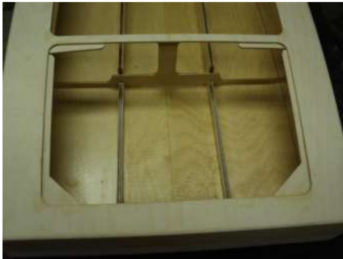
Hatch tongues glued to opening.
