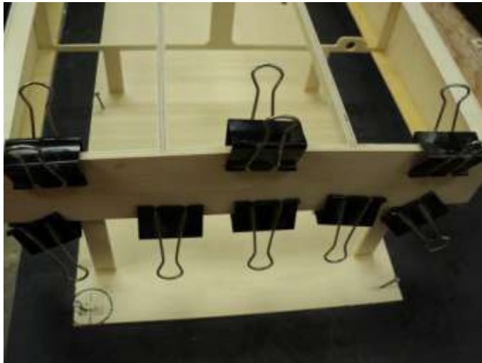
Transom clamped in place.
