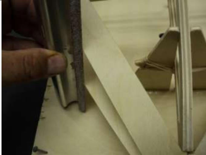
Using sanding block to blend chines.
