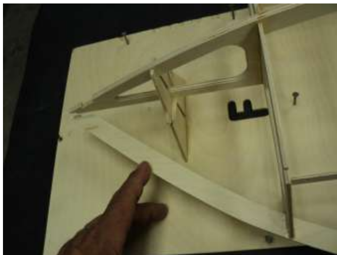
Fitting top chine in place.
