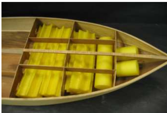
Flotation installed. You will have to leave out some to clear the fuel bag. (Zipkits VBox shown).
