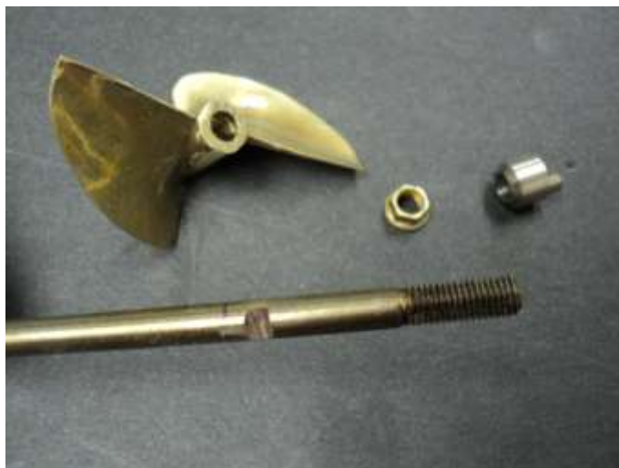
Shaft filed for drive dog set screw.
