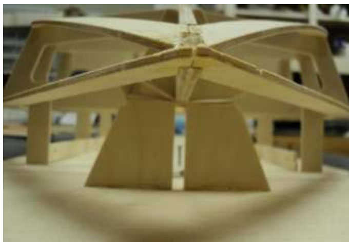
Ant view of the nose. Bottom chine beveled into top.
