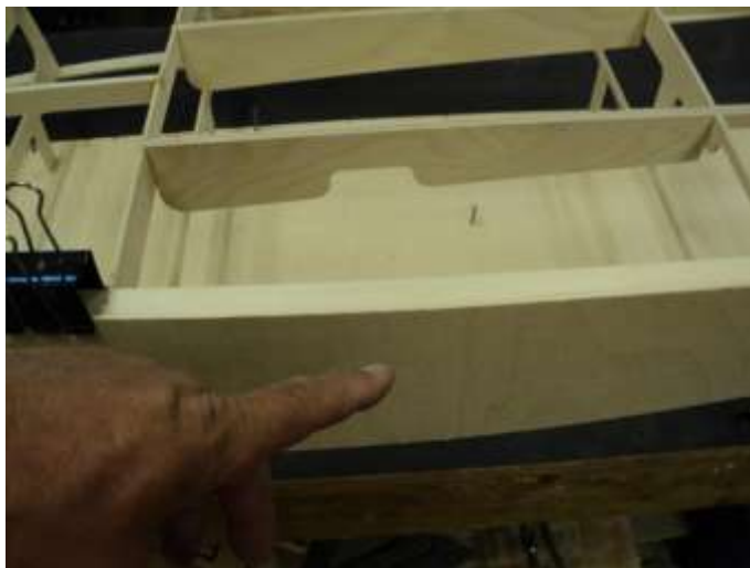
Don't clamp this area until last. Then clamp carefully.
