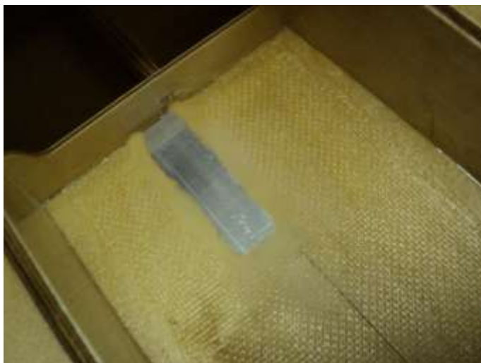
Skeg with epoxy in place.
