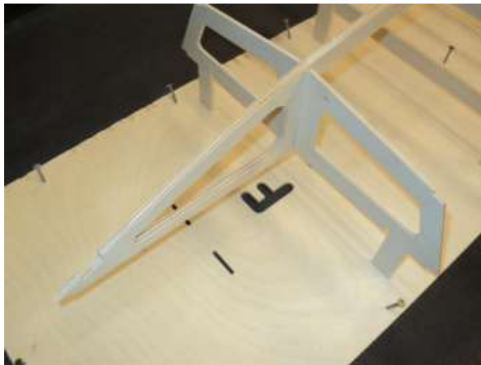
Keel glued to the face of BH 1. Be sure it's square.
