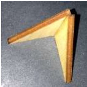
Rudder tube square tool.
