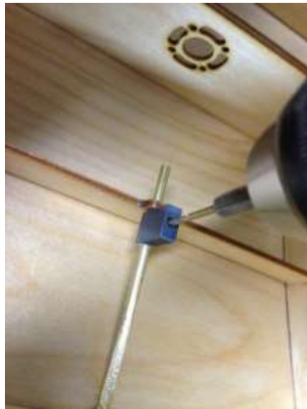
Oiler block being drilled with a 3/32 bit. Be careful.
