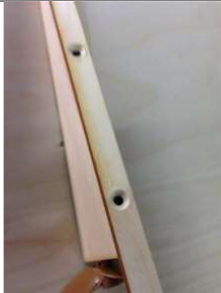
Countersink holes for screws.
