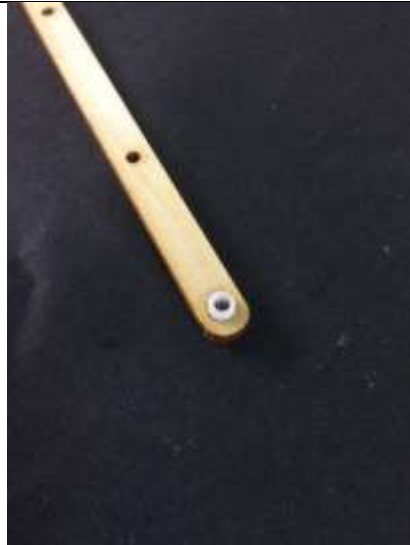
Bushing glued in place.
