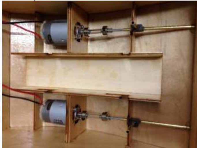
Shafts and couplers in place.
