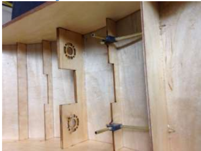
Shaft tubes and oilers glued in place.
