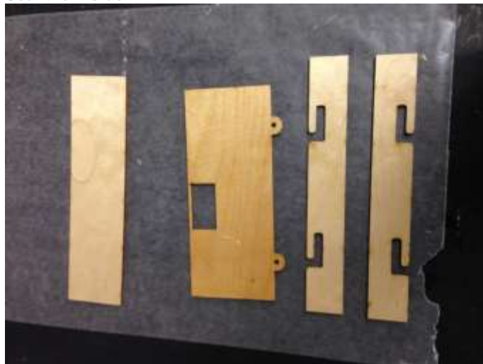
Parts sealed on one side before assembly.
