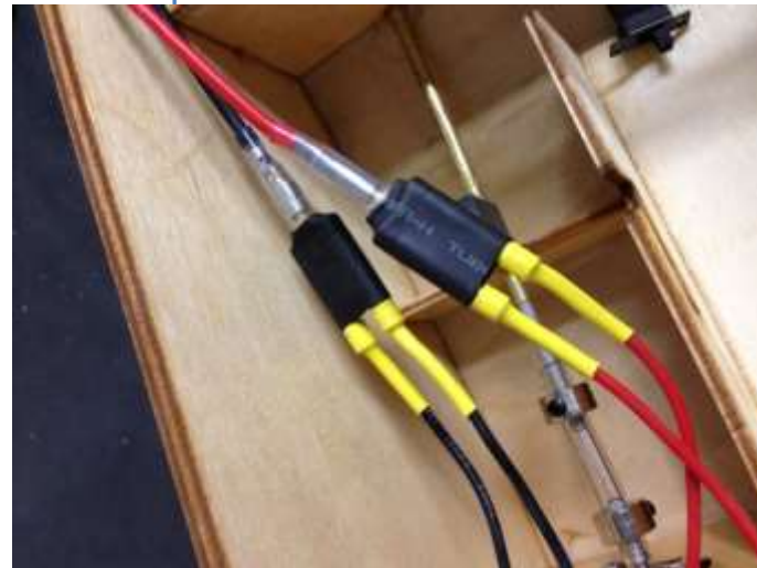
Motors wired in parallel.
