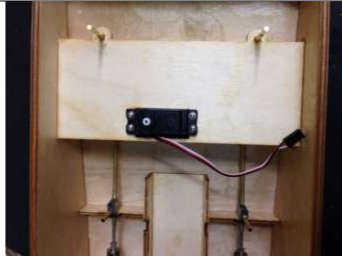
Rudder servo in place.
