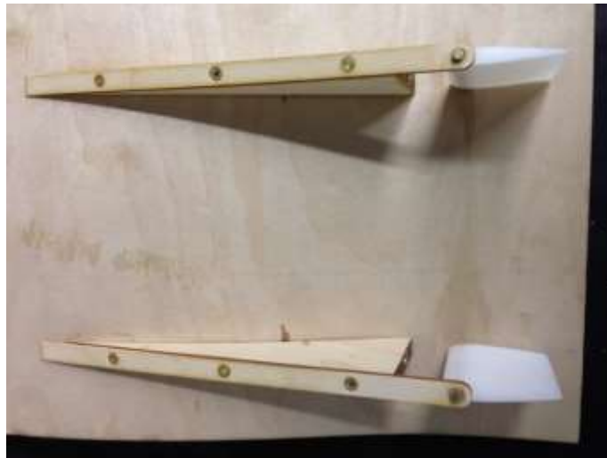
Keel shoes in place. Note how they provide rudder support.
