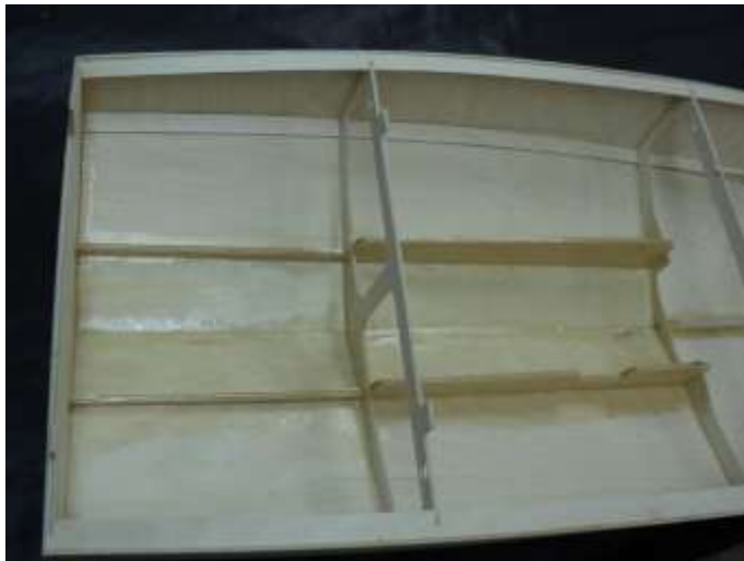
Fiberglass on center seam.
