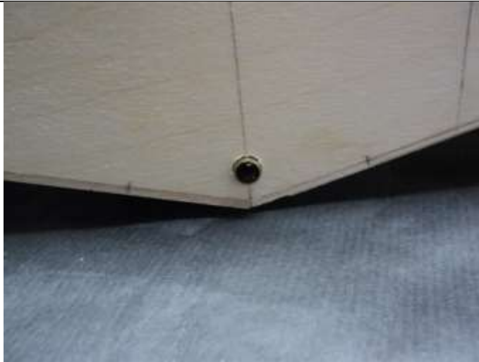
5/16 brass shaft tube in place.
