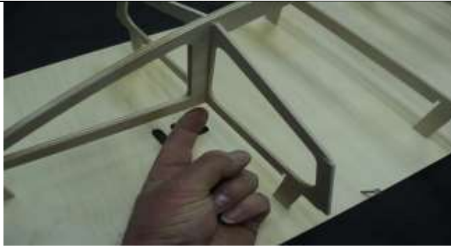
Make sure keel is flush with top of BH1.
