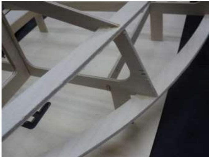
Install chines following angle of bulkhead.
