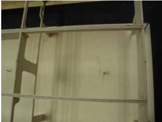
Center marks on bulkheads 4 and 5.
