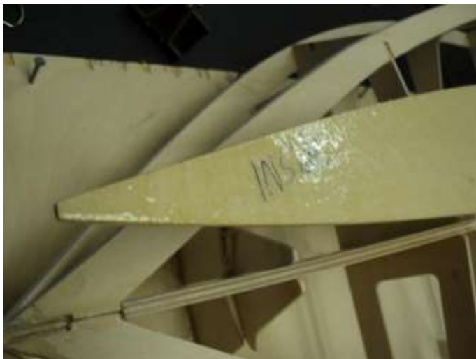
Front of side sheeting coated with epoxy.
