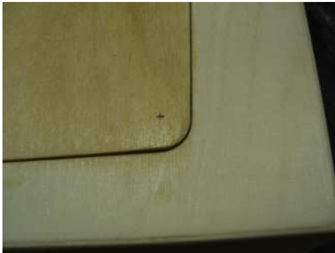
Hole marked for hatch screw.
