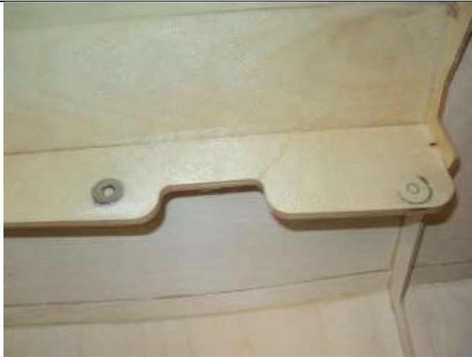
Using washer to mark center holes.
