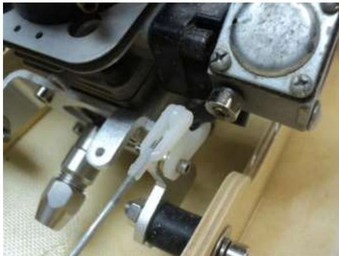
Close up of throttle bellcrank.
