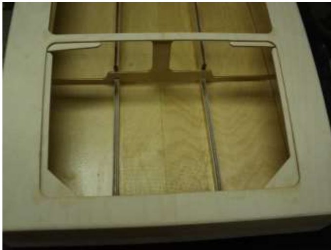
Hatch tongues glued to opening.
