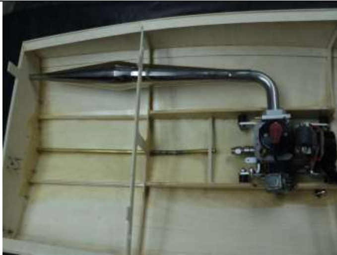
Pipe against transom for marking.
