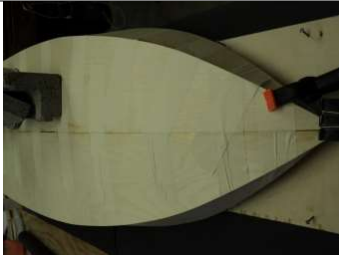
Both bottom halves taped and weighted.
