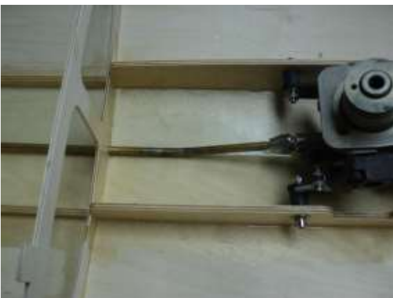
Shaft tube in place over drill bit.
