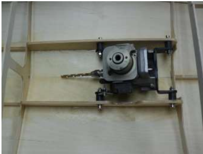
Engine mounted to rails.
