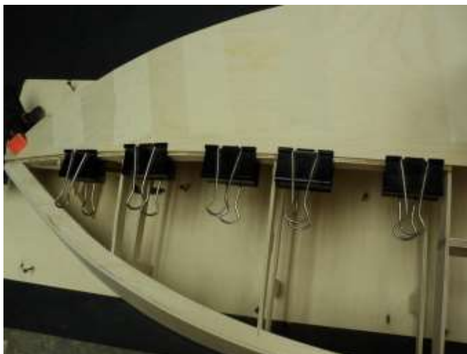
Bottom sheet taped and clamped in place.
