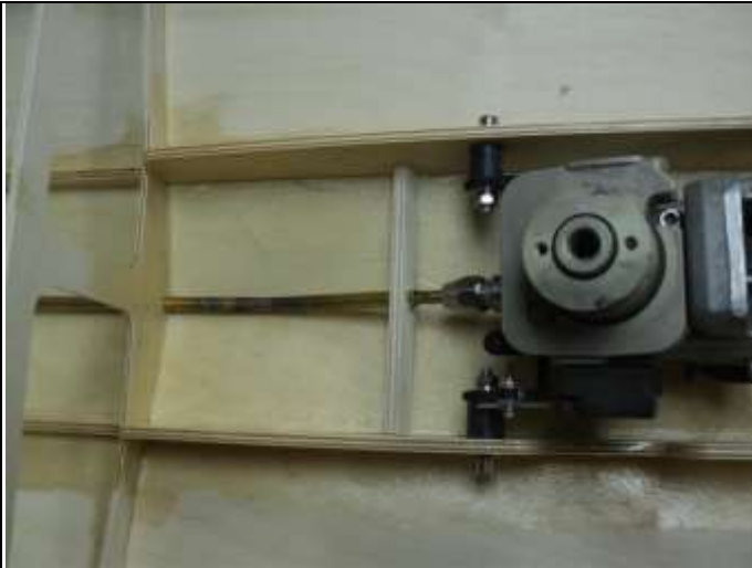
Shaft tube brace installed.
