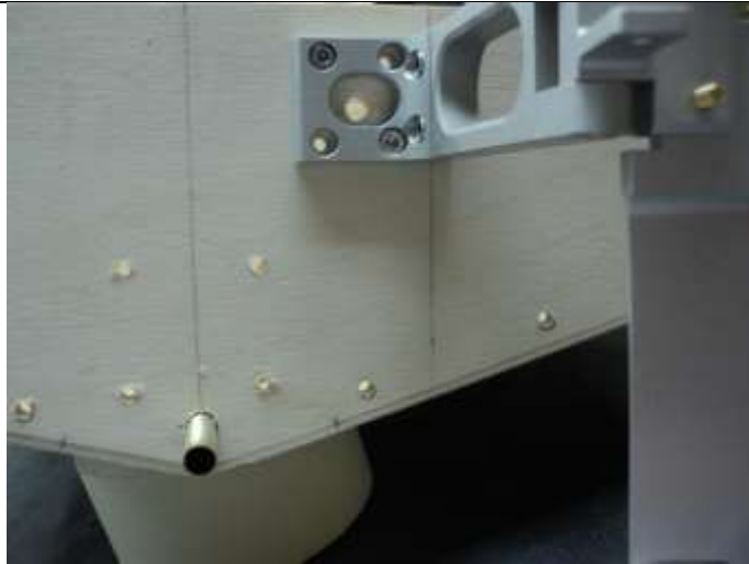
Rudder mounted over pushrod hole.
