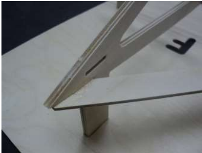
Fitting front of deck chine in place.
