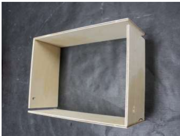
Joining sides. Short sides go between long.
