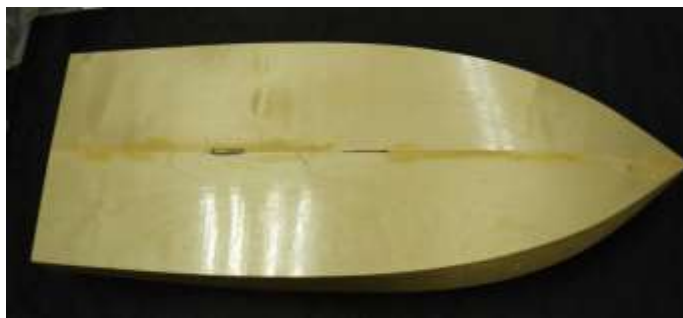
Hull with two coats of clear epoxy.
