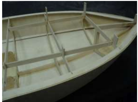
Note how bottom chine matches bottom angle until BH 2.
