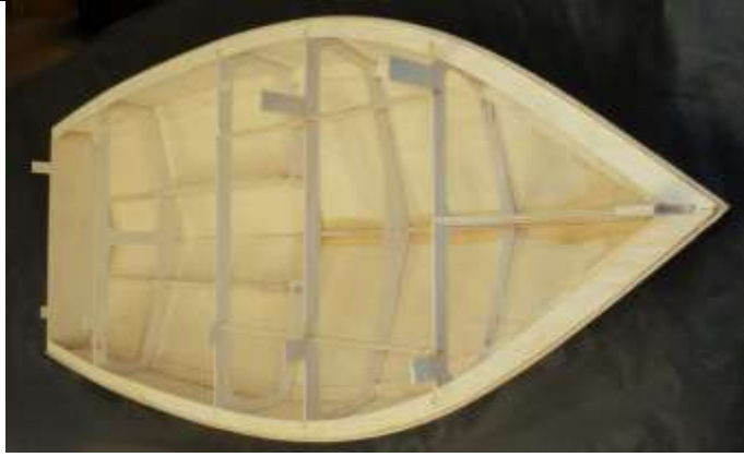
Boat flipped over and off of jig.
