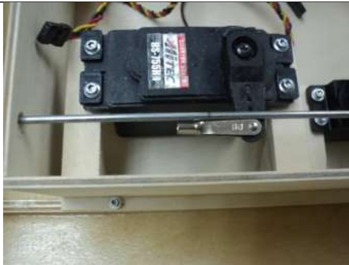
Marking rudder pushrod. Be sure rudder is straight.
