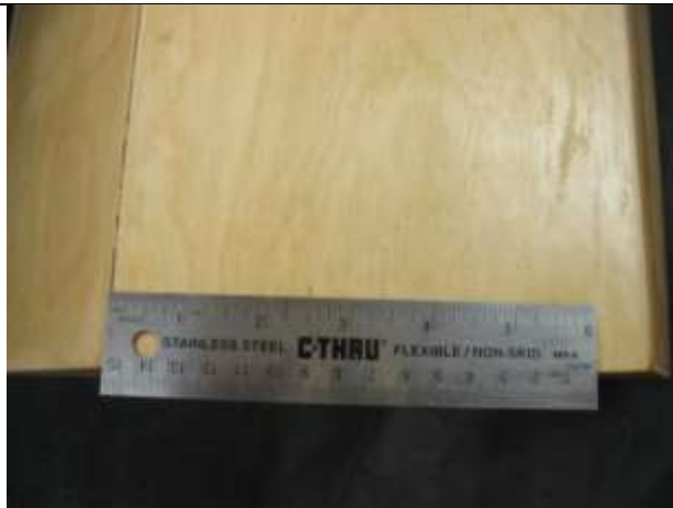
Measure 2-1/2 inches from the keel for strakes.
