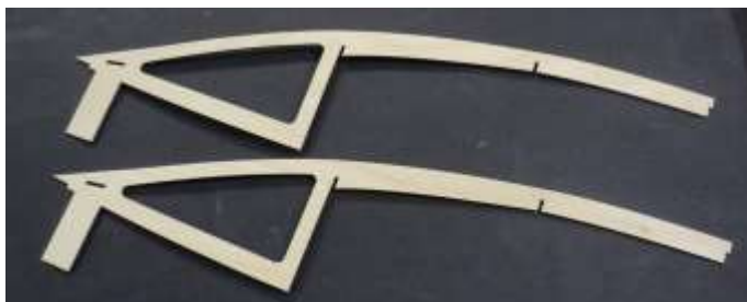
Keel halves before being laminated.
