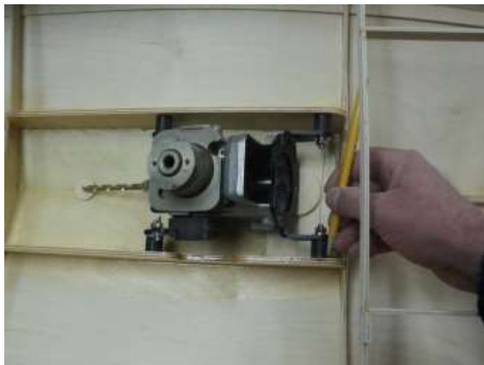
Tracing around rubber mounts.
