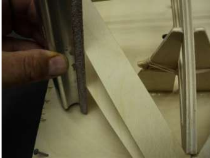
Using sanding block to blend chines. Abox shown.
