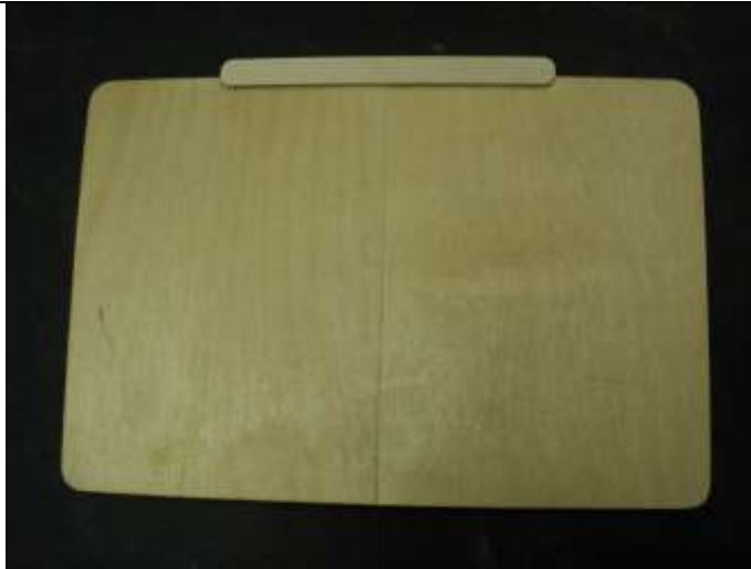
Hatch tongue glued to front of hatch.
