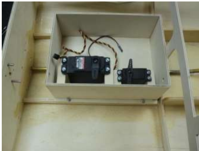
Radio box screwed in place.
