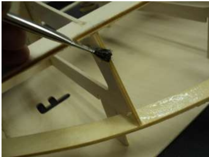
Brushing epoxy onto edges with cut down acid brush.
