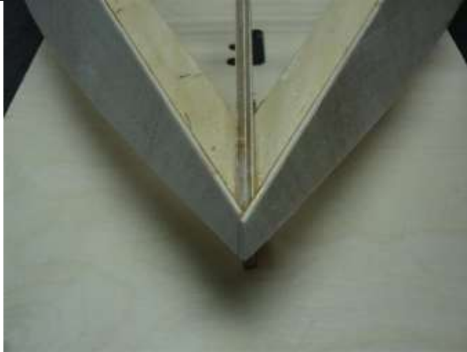
Side sheeting sanded flush at nose. Note overlap.
