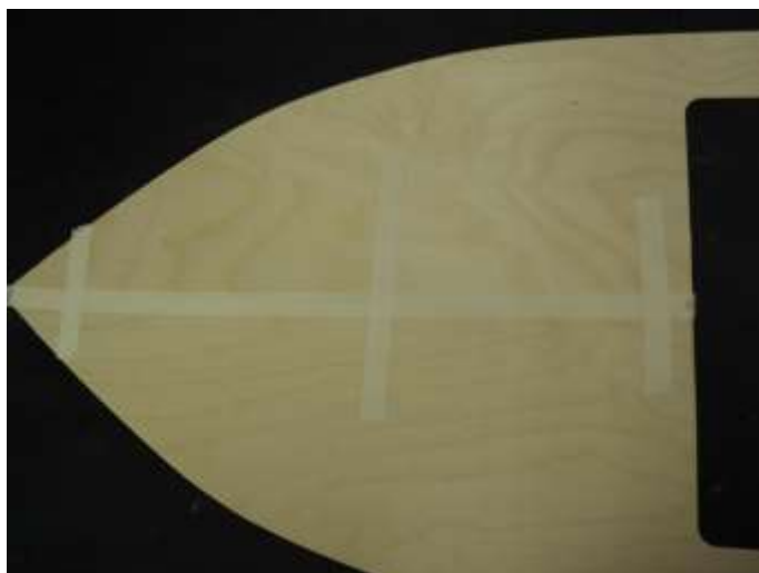
Top deck taped together until cured.
