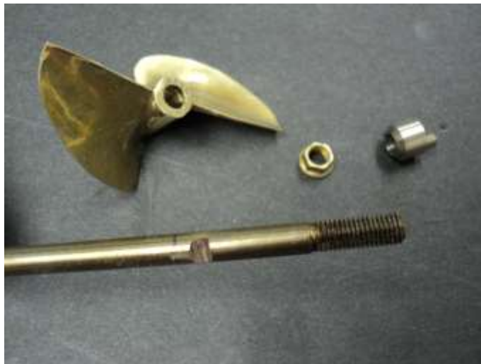
Shaft filed for drive dog set screw.
